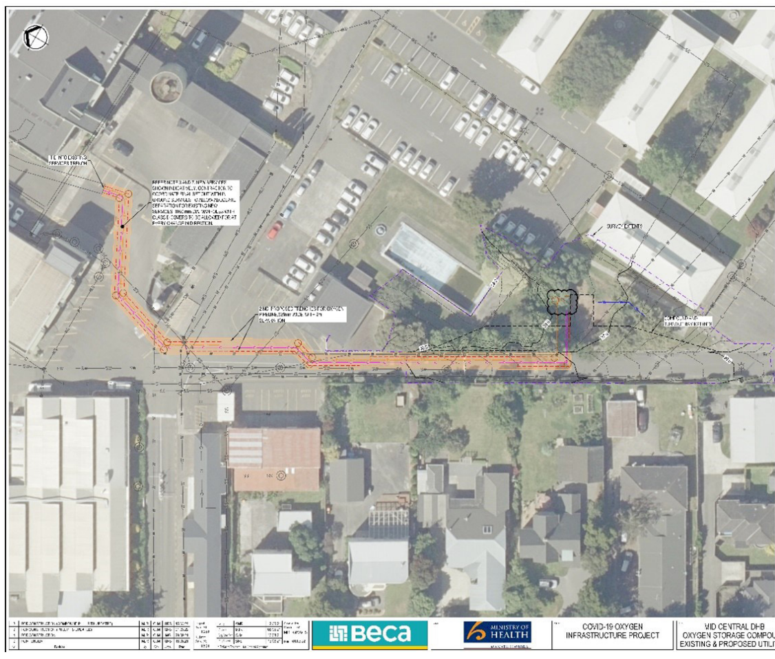
The oxygen ring main plan shows the pipework to be installed over coming months.
